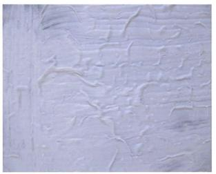
After conditioning the Glass Advanced film was peeled off by hand prior to testing.
